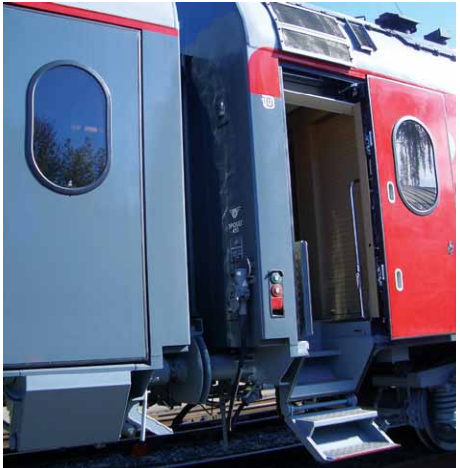
Modern reclining-sliding door for the passenger car
