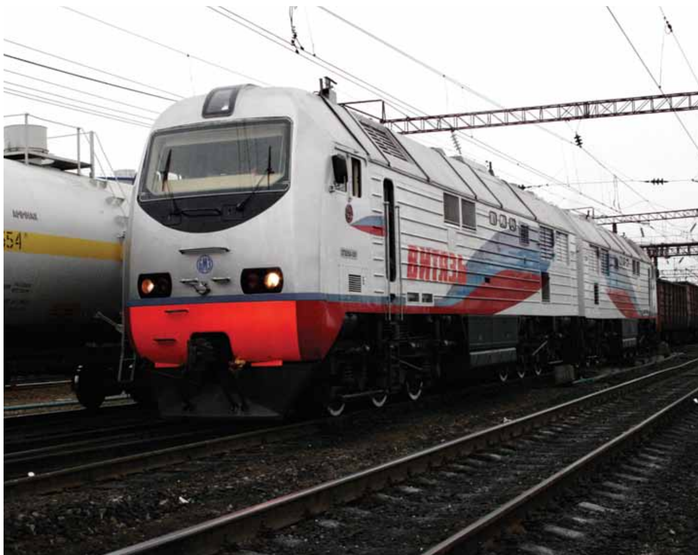
Mainline diesel freight locomotive with asynchronous traction drive 2TE2A Vityaz
