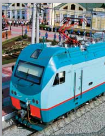
2ES4K Donchak — first Russian freight DC electric locomotive
