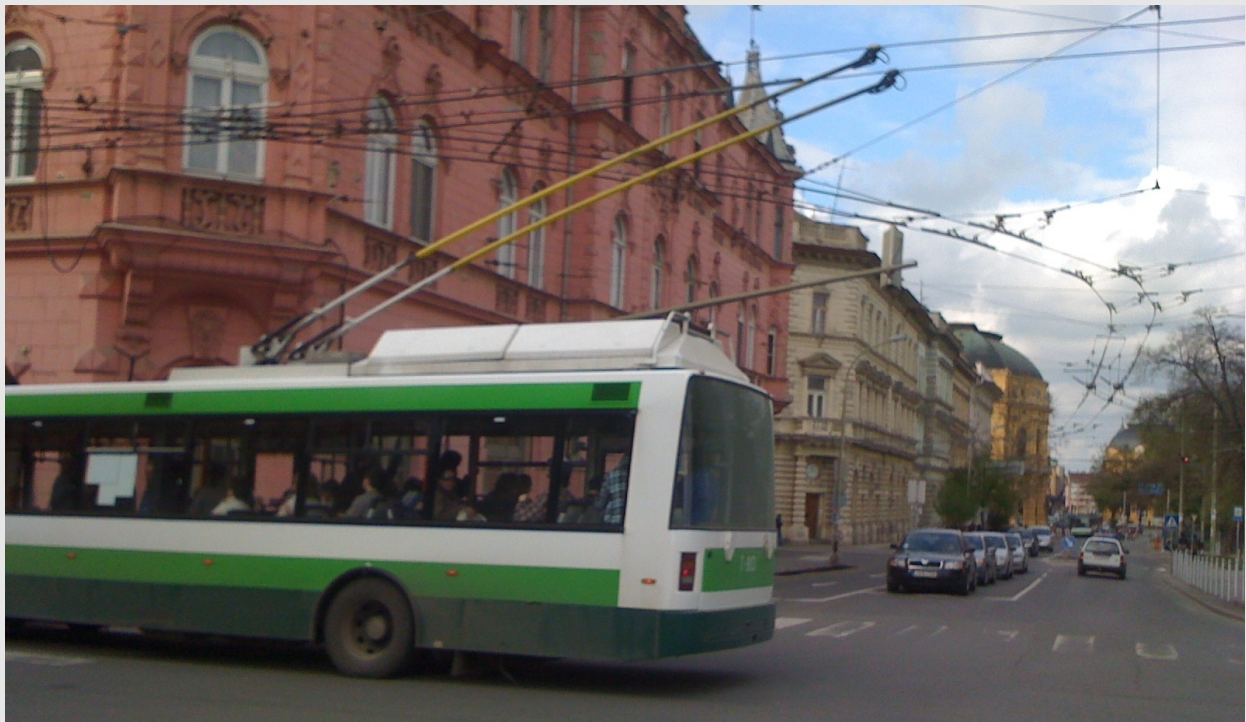
The old catenary at the bridge head with a crossing and a turnout
