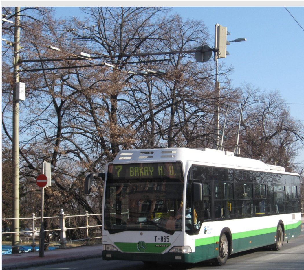
The holding arm for the switch at the bridge head for the turnout, that has no anchoring. Its produces relatively small extra force on the mast, so we could use the existing mast of the traffic-lights. In the background behind the trolleybus one can already see one of the unknown type of rectangular masts that are used on the bridge
