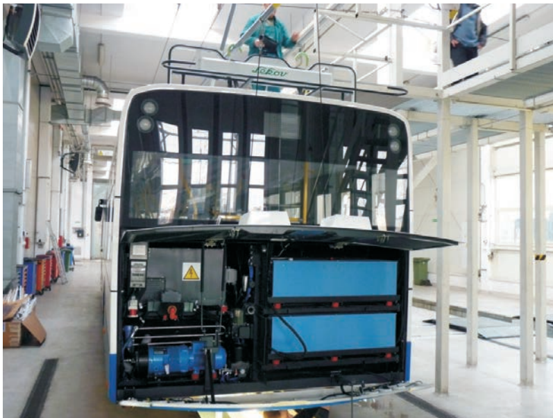
Fig. 2.4. Two modules of nickel-cadmium batteries built into a Solaris Trollino 12M trolleybus in Gdynia in 2009 r.
