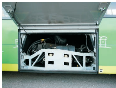
Fig. 4.3. The interior of the traction motor chamber placed between the vehicle's axles (Solaris Trollino 15) Photo M. Bartłomiejczyk.
