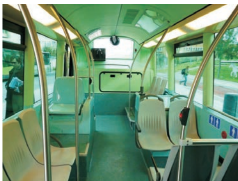
Fig. 4.4. The back part of Cristalis trolleybuses, equipped with AC induction (asynchronous) motors in the hubs – note the wide passage for passengers Photo M. Bartłomiejczyk.
