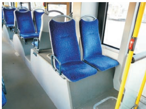
Fig. 4.2. Traction motor chamber placed between the axles, covered with passenger seats (Solaris Trollino 15) Photo M. Bartłomiejczyk.
