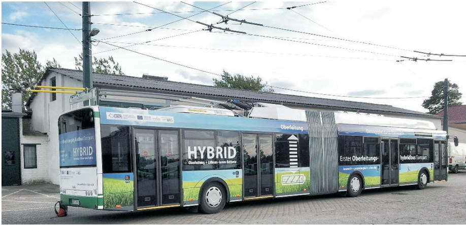
Fig. 9.2. A TROLLEY pilot investment: Europe's first Trolley-Battery-Hybrid-Bus in Eberswalde Source: Barnim Bus Company.
