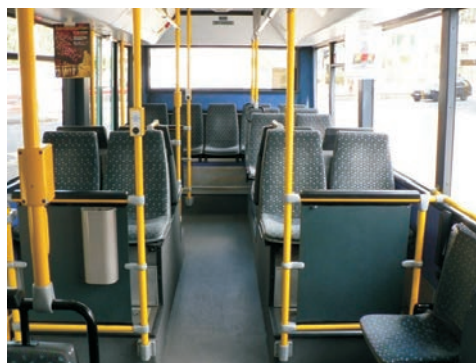
Fig. 4.5. The back part Neoplan trolleybuses, equipped with DC traction engines in the hubs – note the wide passage for passengers. Photo M. Bartłomiejczyk.
