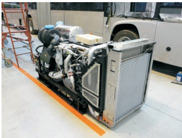
Fig. 2.3. Combustion unit ready for installation in an articulated Breda MenariniBus trolleybus bound for Rome, with an electric motor by Škoda Electric in 2011
