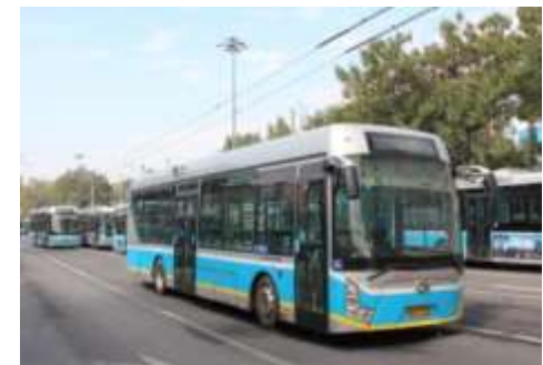
One of BJD-WG120EK trolley converted from battery bus BK6122EV2
