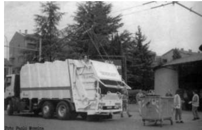
waste trucks with trolleybus technology in Bologna
