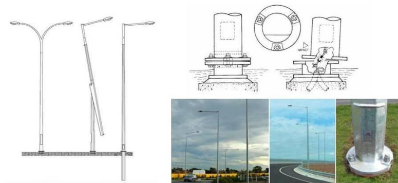
Figura 24: Stâlpi de tip “rupere de la bază” (Source: Department of infrastructure, Energy and Resources: Road Hazard Management Guide, Tasmania, 2014)
