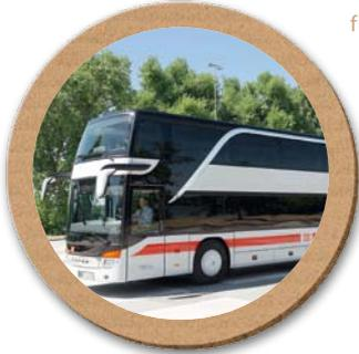
**MANUFACTURER** Daimler AG | **COMMISSIONING** from 2013 | **POWER** 375 kW | **MAXIMUM SPEED** 100 km/h | **SEATS** 74 | **ADDITIONS 2014** 24 | **NO. AS OF DEC 31, 2014** 29
