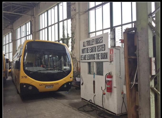
Above: 376 (and all its colleagues) have been earth tested for the very last time. From now on they will either have to be moved using their onboard battery power (for how long that lasts) or be towed by the depot tractor. The electricity to the overhead has been switched off.
