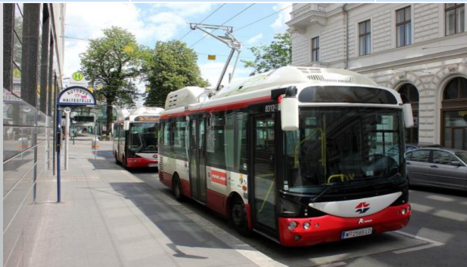
Siemens-Rampini charging (Wien – from tram infrastructure, Pardubice – from trolley infrastructure)
