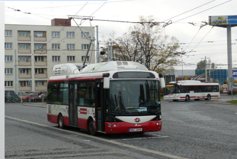
Siemens-Rampini charging (Wien – from tram infrastructure, Pardubice – from trolley infrastructure)
