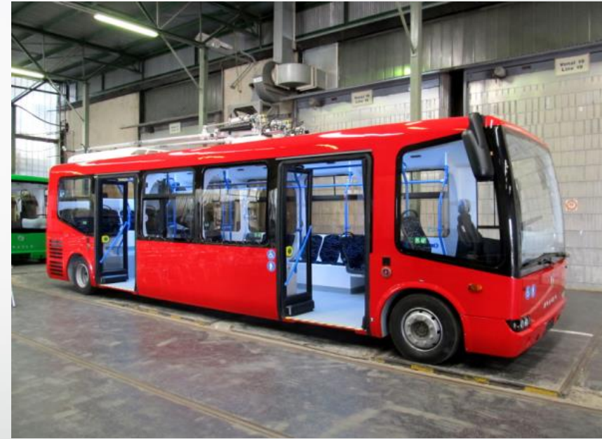
Modulo composite frame trolleybus (Evopro group)
