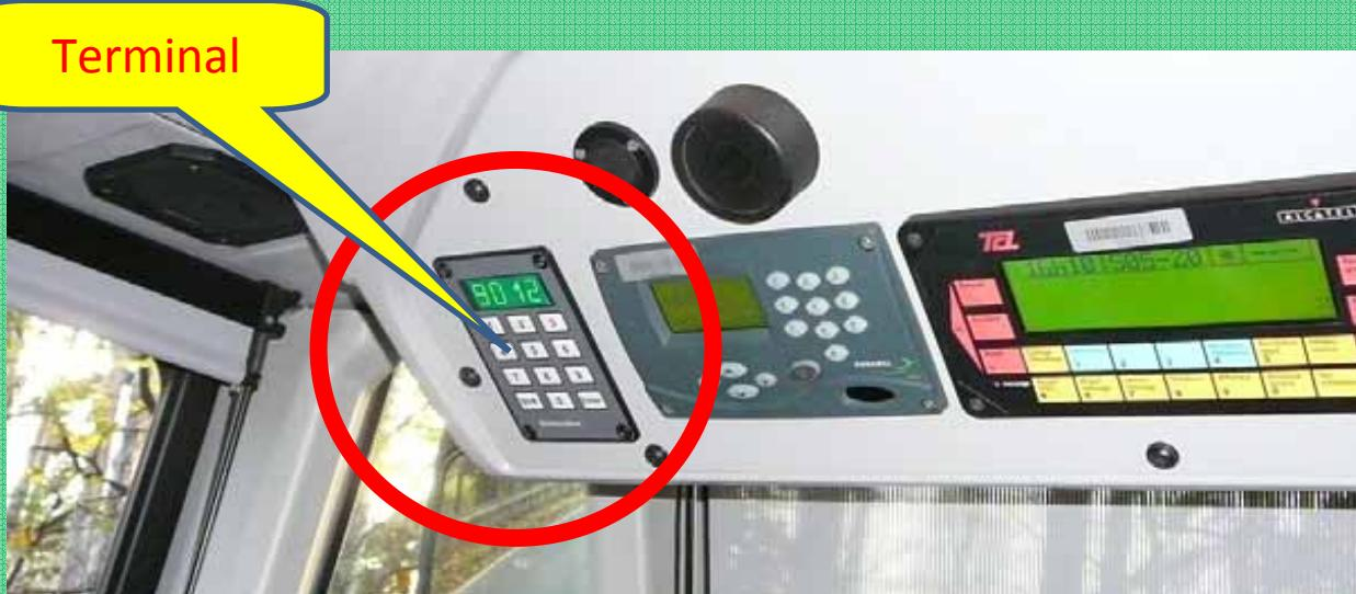
Vehicle **terminal** is possible to connect with a board computer.
