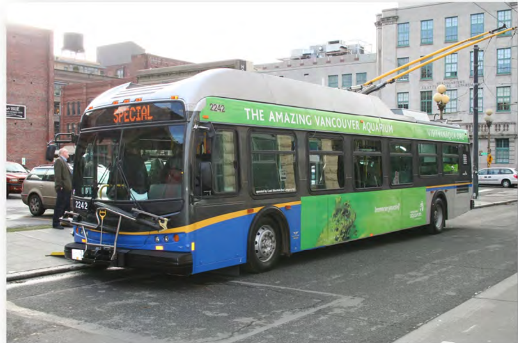
Exhibit 1-5. New Electric Trolley Bus Operating in Vancouver, B.C.
