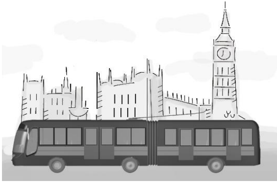
Figure 3. Trolleybus using his energy backup: batteries, ultracapacitor or thermal engine. Ideal to avoid overhead line where is undesirable.
