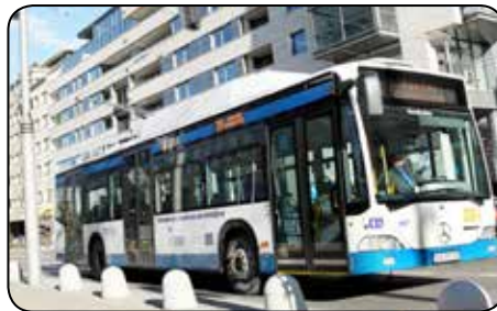
Diesel bus converted into a trolleybus in Gdynia
