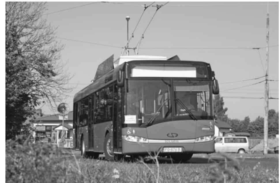
Fig. 3. New type of low floor trolleybus Solaris Trollino with electric drive from polish company Medcom
