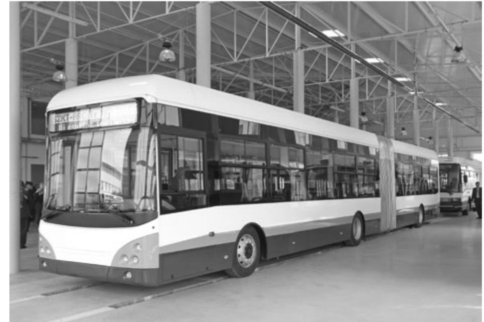
Fig. 5. New type of articulated low floor trolleybus ARC trolleybus assembled at the depot in Szeged
