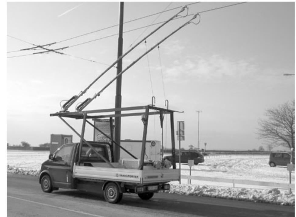
Fig. 5. In February 2005 this de-icing vehicle was delivered
