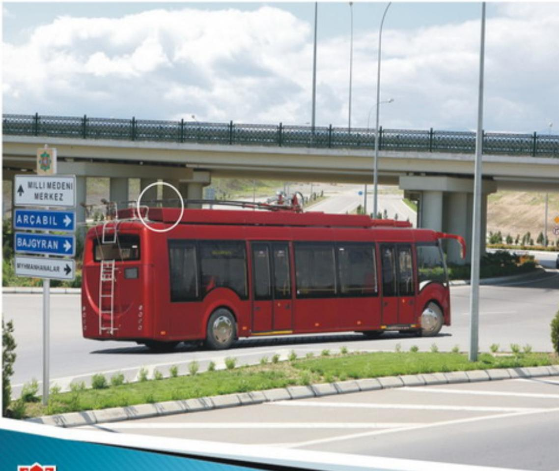
Trolleybus is equipped with modern accumulators which offer the possibilities to move without being connected to the high voltage system up to 5000 m. These options confer to the trolleybus capacity to operate in the sectors without high voltage system.
