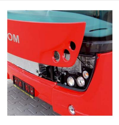
Easy access when lights replacing
