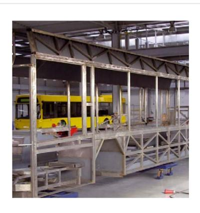
Bodywork frame of stainless steel = long life span period of the vehicle
